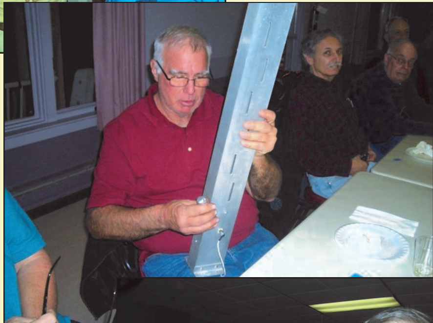
Warren inspects a 13? Cm slot antenna.
